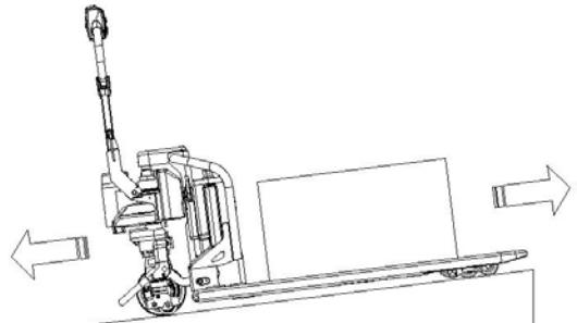
Connect the battery plug (11), insert the key and turn the key switch (13) clockwise, move the tiller to the operating one ('F', fig.9).
