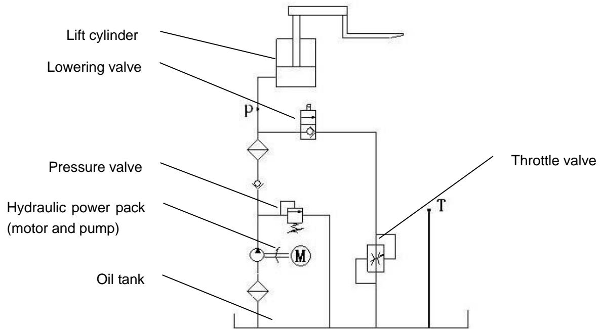
Fig. 16: Hydraulic circuit
