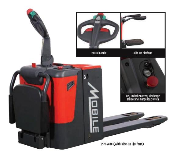
The ESPT44N self-propelled pallet truck is designed for heavy duty lifting and transporting applications. These units feature full electric lifting and self-propelled movement with the option of a "ride-on' operator platform, enabling safe and more efficient load handling, particularly in long-distance warehouse applications.
