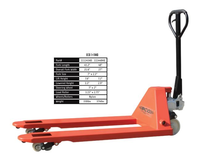
The ECO I-11HD Heavy Duty Pallet Truck is designed for extra heavy duty applications. It offers the same durability as the ECO I-55, but reinforced to handle loads of up to 11,000 lbs. Like the standard ECO I-55, the ECO I-11HD offers 200 degree handle pivot for exceptional maneuverability in compact areas; comes with standard polyurethane wheels and heavy duty load rollers;
