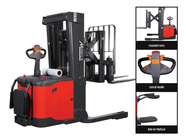
The ECO RTS self-propelled stacker is designed to handle a wide variety of heavy-duty applications. Able to lift loads up to 3,000 lbs to a maximum height ranging from 114.1" - 216.5", this state-of-the-art stacker also extends loads to a maximum of 22.4".
